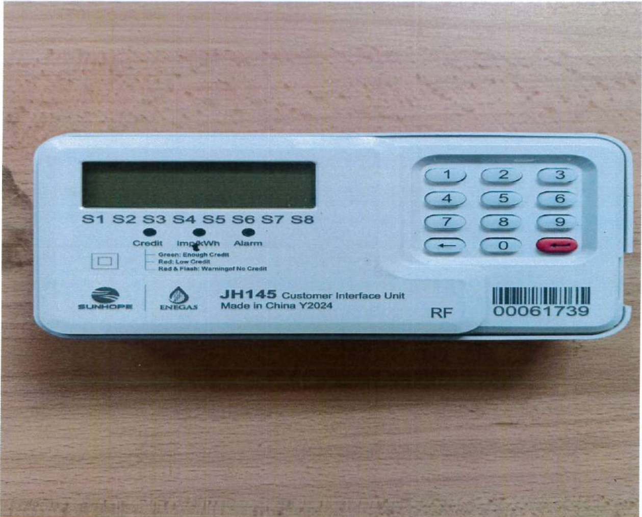
Photograph of HANGZHOU SUNRISE TECHNOLOGY CO., LTD & ENEGASLONGMEN JV LTD Three Phase Smart Prepayment Meter Customer Interface Unit (CIU)
