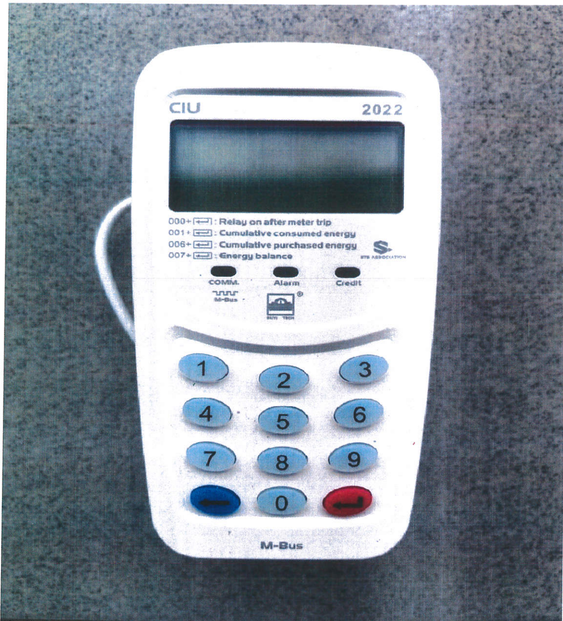
Above is a photograph of BUWI TECHNOLOGY CO. LTD & ENEGASLONGMEN JV LTD Three Phase Four Wire Smart Prepayment Energy Meter Customer Interface Unit (CIU).
